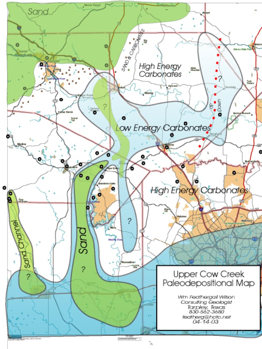
FIGURE 23: - REGIONAL FACIES COW CREEK MAP. THE BLUE AREA DEPICTS LOW POROSITY AREAS, WHILE THE WHITE AREAS DEPICT HIGH ENERGY POROUS AREAS. THE GREEN AREAS REPRESENT QUARTZ SAND FACIES.
