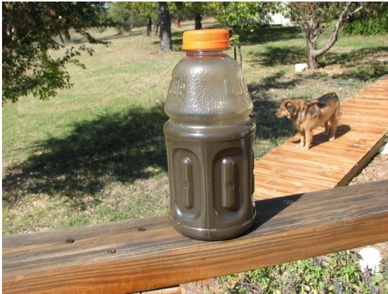
FIGURE 39: - HGCD-MW-12 OIL AND WATER EMULSION.
